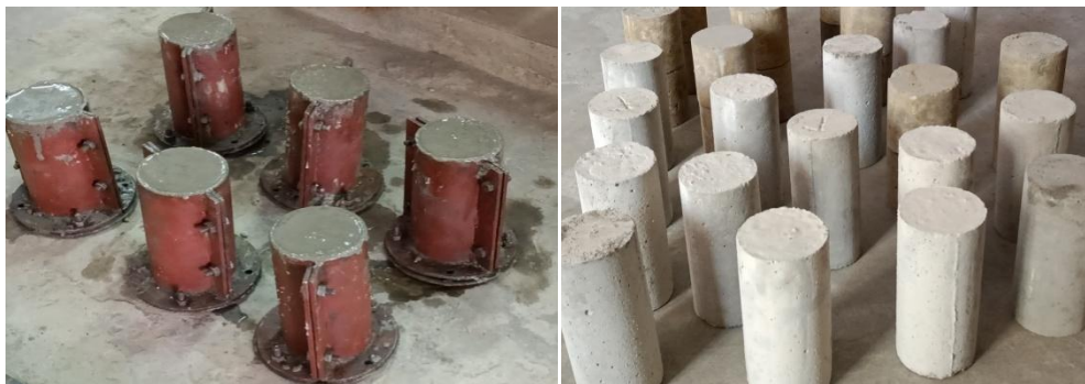
Figure 5.1 Casting of specimens
